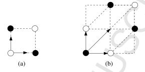
Figure 2: Non-unique reconstructions from (a) two and (b) three projection directions. Black and white circles denote two possible solutions with identical projection data; projection directions are indicated by arrows. Similar examples exist for any prescribed set of projection directions.
