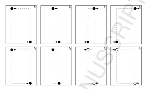
Figure 3: An example illustrating that PTV may track particle paths that do not exist but which are consistent with the data.
