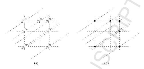
Figure 1: A two-dimensional example for three projection directions (signal-recording lines indicated by dashed lines). (a) The grid  $G^{(t)}$ , and (b) a possible solution  $\underline{\vec{x}}^{(t)}$  representing a set of particles that are consistent with the projections (black and white dots corresponding to  $\xi_i^{(t)} = 1$  and  $\xi_4^{(t)} = 0$ , respectively).
