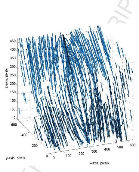
Figure 5: Reconstructed velocity field obtained by tracking 500 particles in 3D over 50 frames. The arrows indicate the velocity vectors at the corresponding positions in the volume. More than 98% of the velocity vectors are correctly reconstructed.
